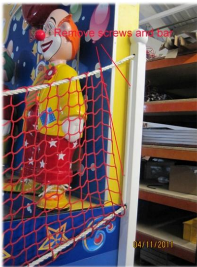
12. Fasten the side nettings in position.
